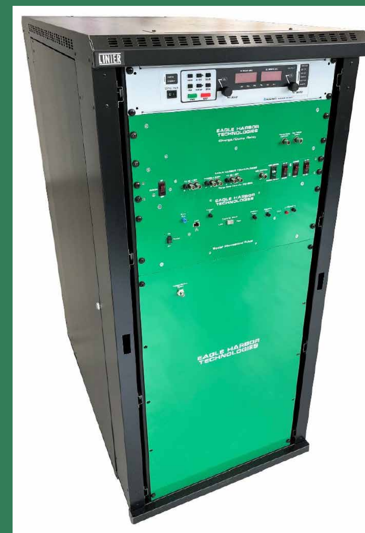
Left: Bipolar microsecond pulser with capacitor bank, charge/dump system, and DC charging supply. Right: Output voltage measured across a 70 \Omega load, 3 kV charge, 50 \mu s (top) and 500 \mu s (bottom) pulse width for both the positive and negative pulse, no dwell between pulses.
